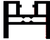
TİJLİ DİKEY BAZA VERTICAL BASE WITH ROD Stok : 7 mt Ağırlık / Weight: 0,715 Kg/m
